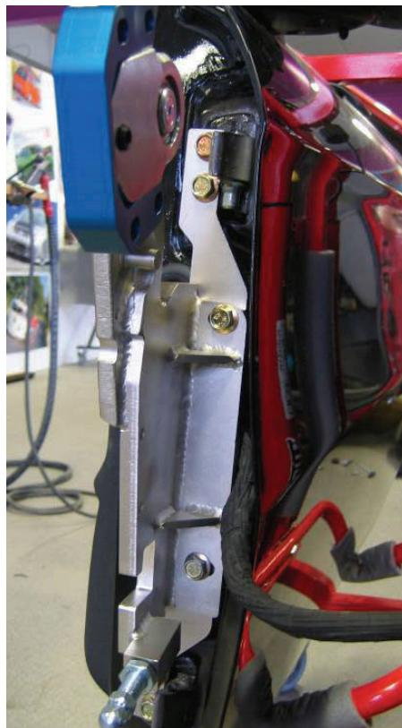
14.) Now you can attach the LSD swing arm to the door plate with the supplied bolts.
