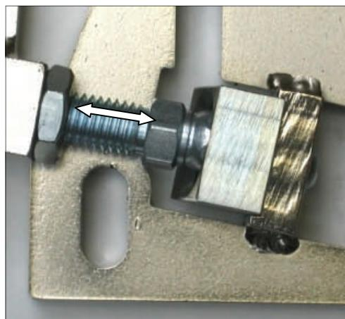
16.) Position the lower adjustment screw (1) in that way, which the door closes in the middle position.
