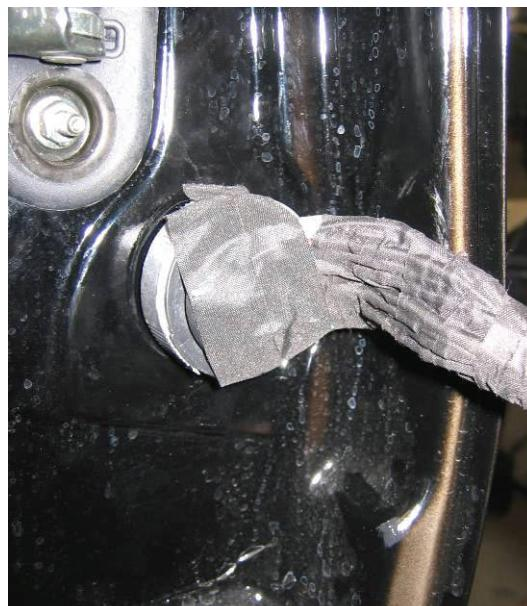
11.) Afterwards please seal the plug-and-socket connection with the supplied chassis glue and insulation tape for protection.
