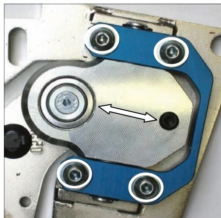
17.) Attach the swing arm to the chassis plate with the 4 included Allen bolts and adjust the door via moving the swing arm to chassis plate adjustable connection (2) mount with horizontal door gap adjuster (2) in the right or left direction.
