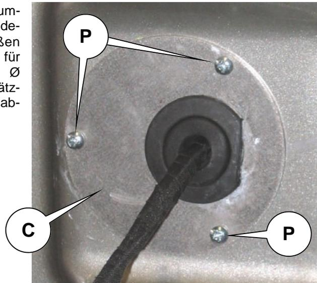
2.) The original wire harness lead-through hole can be covered with the supplied wire cover plate (**C**) self tapping screws (**P**) and sealed with the chassis glue (drilling Ø 2,6 mm/0,1" holes are required)
