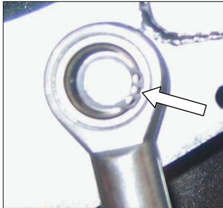
16.) Hang in the gas damper (L) on the fitting point of the swing arm. Secure it with the supplied security ring, by means of needle-nosed pliers.
