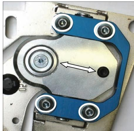
8.) Attach the swing arm **(N)** to the chassis plate **(O)** with the included Allen bolts (4x) and adjust the door via moving the swing arm to chassis plate adjustable connection **(2)** mount with horizontal door gap adjuster **(2)** in the right or left direction until gap measurement is like original.
