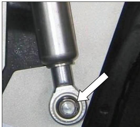
17.) Carefully pivot the door up and hang in the gas damper (L) at the fitting point of the chassis plate. Secure it also with the supplied security ring.
