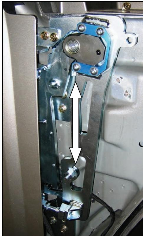
9.) Adjust the height of the door by moving the chassis plate **(O)** vertically. You might have to loosen bolts **(E)** on the chassis plate to do this.
