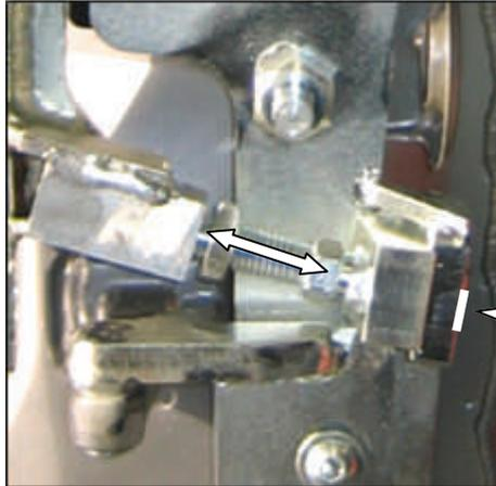
7.) Position the lower adjustment screw **(1)** in that way, which the door closes in the center position.
