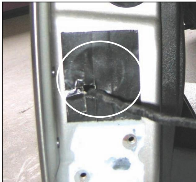
4.) After extending the wire harness please route it as shown in the picture then wrap it fully with the supplied insulation tape.
