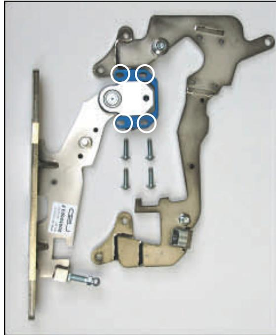
1.) Disassemble the swing arm (**N**) off the chassis plate (**O**).
